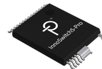
Figure 2. High Creepage, Safety-Compliant InSOP-T28D Package.
